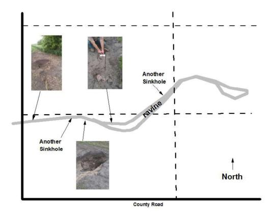
Thick, black lines represent the southwest boundaries of Drainage District 167 in Harding County, IA. Thick gray lines represent the approximate location of the two 8-inch tiles that comprise the main drainage line for the district.
